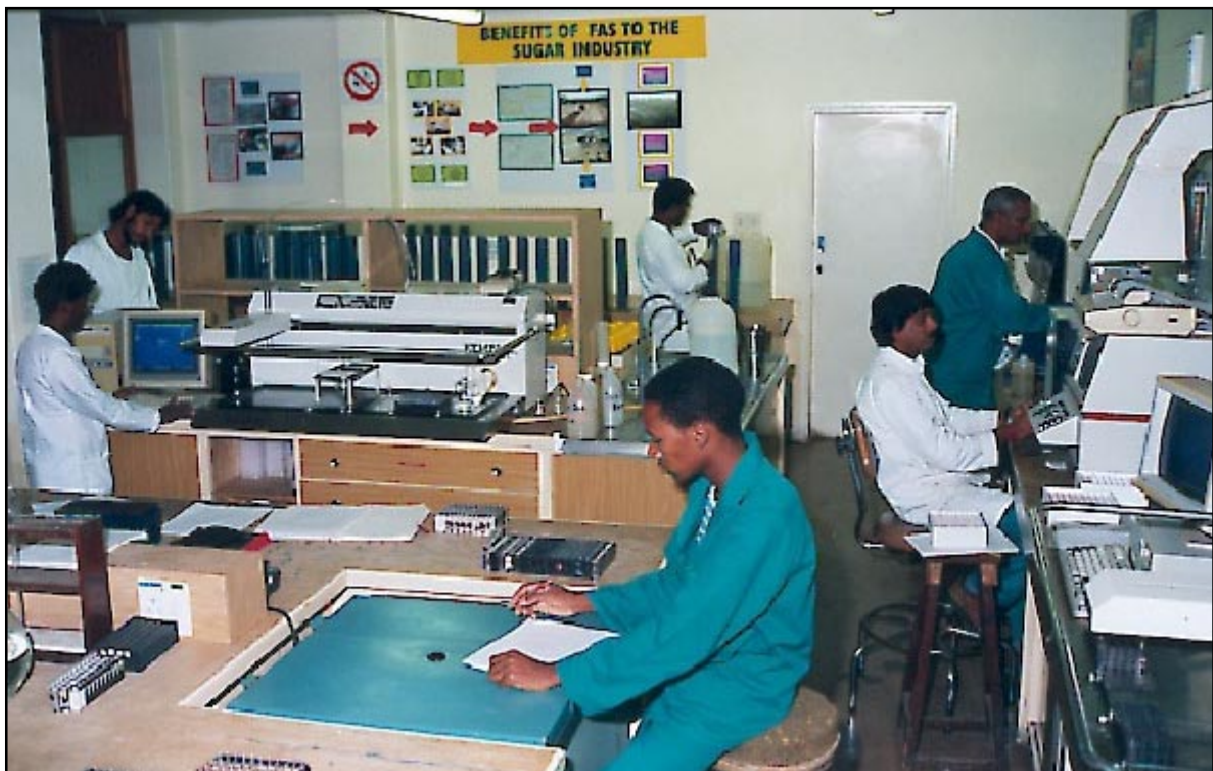
Portion of the FAS laboratory at Mount Edgecombe, showing (front) centrifuge, (back left) Kemble sample processor and (back right) AA spectrometer.
