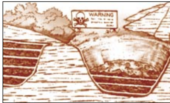
Layers of waste covered with lime, household waste and compost.
